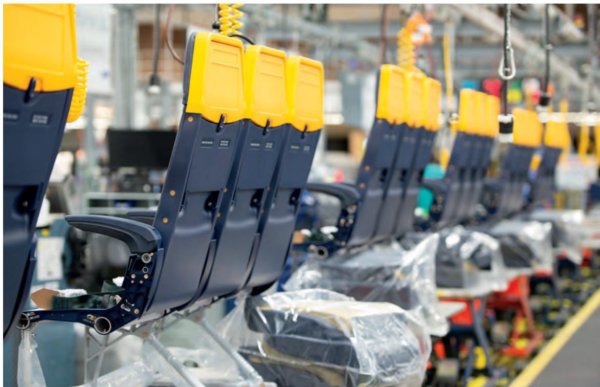
Final assembly of economy-class seats. © Frank Rogozinski/CAPA Pictures/Safran.
